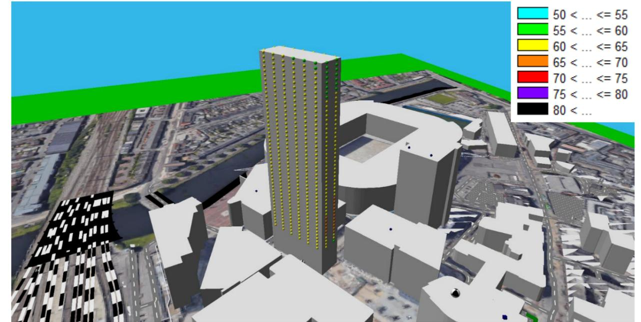
Figure 4-2 - Predicted façade noise levels (dB,  $L_{Aeq}$ ), night time, eastern view
