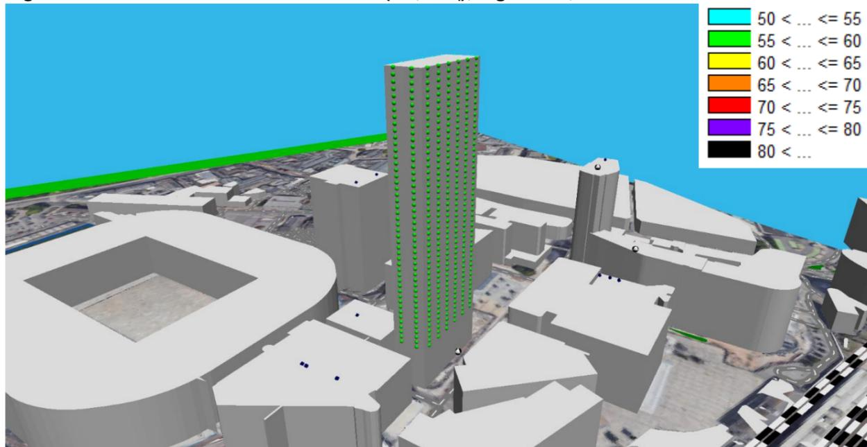
Figure 4-6 - Predicted facade noise levels (dB,  $L_{Aeq}$ ), night time, northern view
